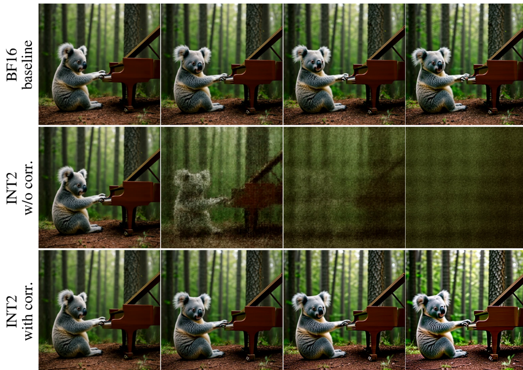
Figure 5. Additional qualitative comparisons on MAGI-1 for two different prompts. Columns show successive frames from the same generated video. From top to bottom in each panel: BF16 baseline; INT2 asymmetric QuaRot+RTN KV-cache quantization of both keys and values; same quantized setting with our correction.
