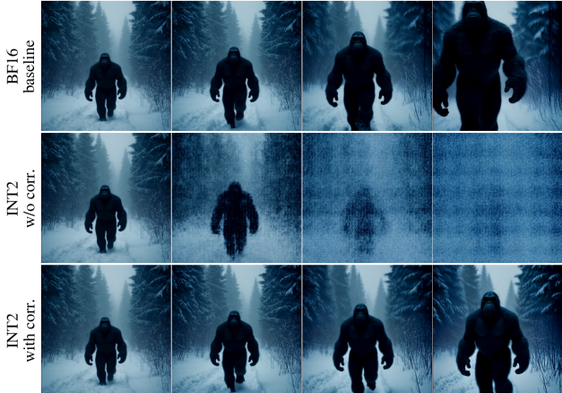
Figure 1. Qualitative comparison on MAGI-1. Columns show successive frames from the same generated video. INT2 QuaRot+RTN KV-cache quantization destroys subject and scene structure, while our correction substantially restores BF16-like visual quality and temporal consistency.
